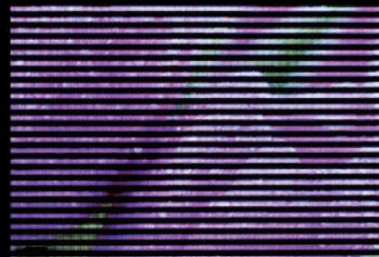
Low refresh rate cause horizontal lines
